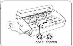
put in suitable paper, adjust the creasing pressure and feeding pressure. Different paper with different creasing pressure.
