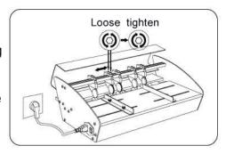
4. adjust the right and left postioning according to the paper size, the scale only for reference, you can fine adjusting the specific direction.
